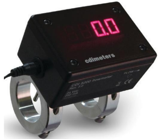
The CDI 5200 clamps onto a pipe, with two flow-sensing probes projecting into the pipe through 3/16-in. drilled holes. It seals directly to the pipe; no cutting or welding is required for installation. Because each flowmeter is made and calibrated for a specific size of pipe, the digital display indicates flow directly, with no setup or adjustment.
